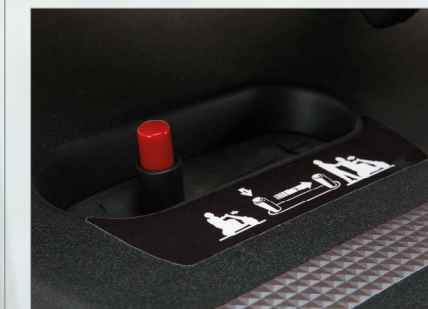
Two-step disengaging lever to prevent free-wheeling
